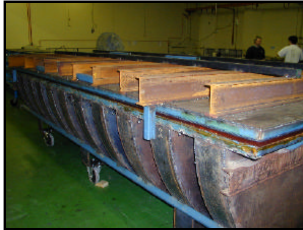
Figure 6: Vacuum chamber/mould used for lamination
